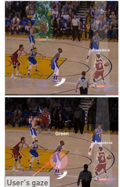
Fig.4 IBALL automatically visualizes the in-game data of important players (Top) and adapts the visualizations based on the context and user's gaze (Bottom).
